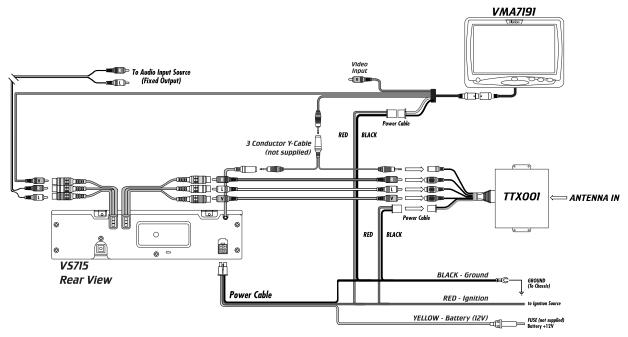
Figure 14. TTXOO1 Wiring diagram for VS715.
